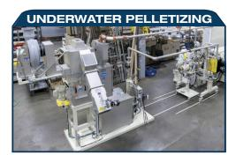
PTi provides options for underwater pelletizing for applications that may require it (i.e.: high melt PP, PET, PLA, PA, etc.) as well as for customer preferences.
