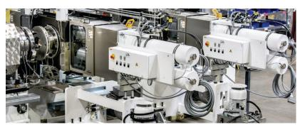
PTi offers several 'recycling duty' polymer filter options, including 'extreme duty' sequential, 4 cavity, dual bolt, back flushing styles.
