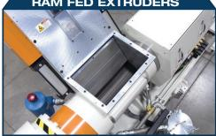
PTi reclaim extruders are available with reciprocating pneumatic Ram Feeders used for boosting machine performance for low bulk density applications, including foam, film, fluff and shredded materials.
