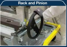
Rack and pinion design, along with a large hand wheel, allows single person die splitting with ease
