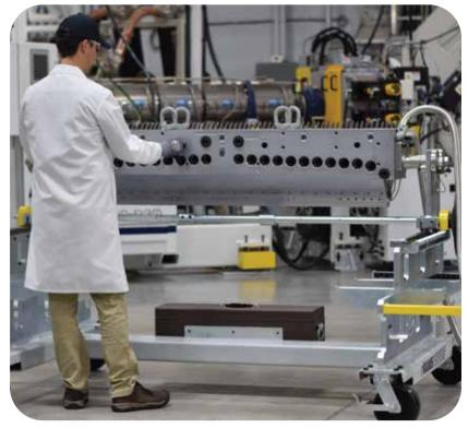
Die handling requires customer supplied lifting/rigging equipment (not included)
