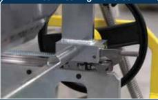
Easy glide linear bearings for precise traverse with hold-open lock to secure positioning
